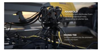
2. The manifold precisely mixes product concentrate with air and a low volume of water; product is then precisely monitored and delivered to each row.
