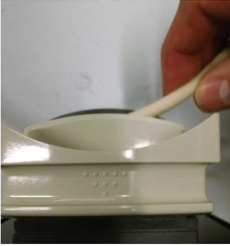
5. Lay the replacement tube into the jaws of the pump. The tube should be approximately centered on roller.
