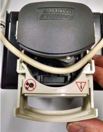
6. Gently close the jaws making sure the tube is centered in the V notch of the jaw cover.
