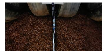
4. The foam solution is applied after seed placement and just before rows close to ensure on-target, dust-free, drift-free application.
