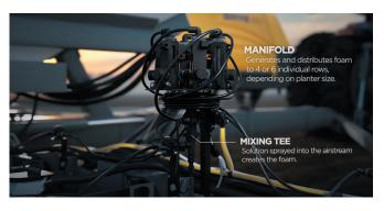
2. The manifold precisely mixes product concentrate with air and a low volume of water; product is then precisely monitored and delivered to each row.
