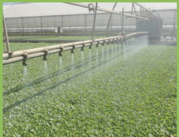
Transplant tray drench application of Verimark insect control using traveling spray boom.
