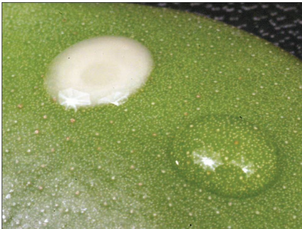
The clear liquid on the leaf surface is a herbicide powered by Solumax®. It is completely dissolved into a clear solution. The DF herbicide is cloudy because its particles are merely in suspension.
