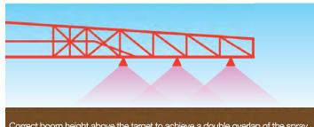
Correct boom height above the target to achieve a double overlap of the spray.
