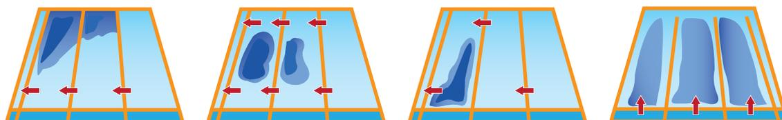
Left: Illustration of bays being filled independently from the supply channel eliminating accumulation of dissolved salts and herbicide.
